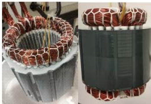
Fig. 1 Motor stator coating by dip and bake method
